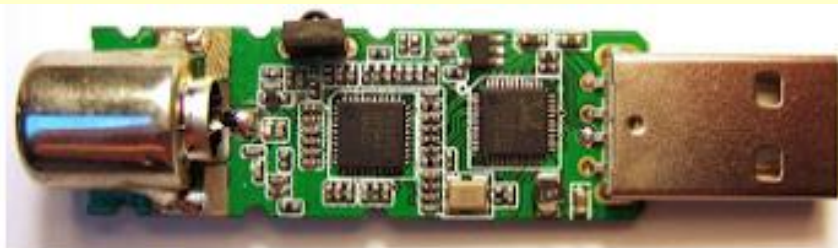
A Terratec Cinergy T Stick Black rev.1, with the FC0012 which is not suitable for GPS
