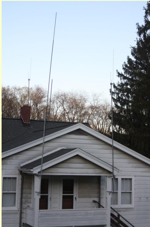
2 meter/440 and 6 meter J-poles. 6 meter dipole is homebrewed.
