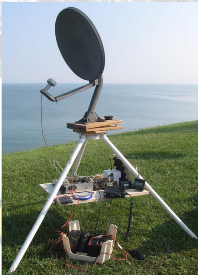
Dish-Tripod with SMA-LNB feed using an Adams-Russell Low Loss Instrument Cable To The 10 GHz Transverter.
